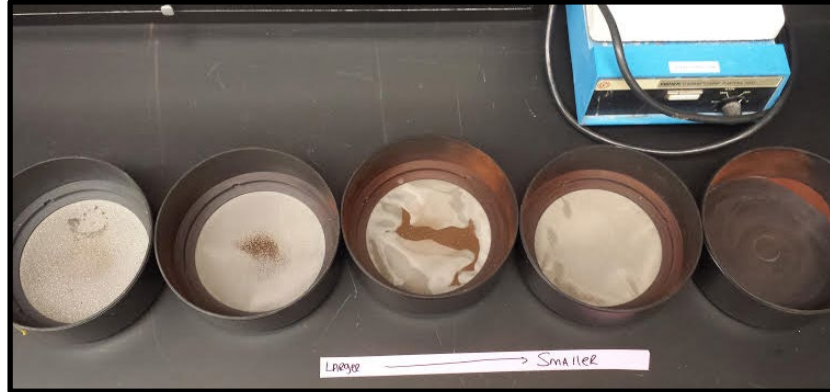
Fig. 5. Sieves used to ensure the ferrihydrite is uniform in size. The smallest sieve only allowed particles less than 125- \mu\text{m} to pass through. Those particles were used in the subsequent experiments.
