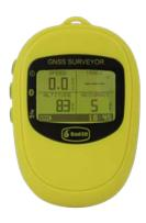
The Bad Elf GNSS Surveyor is a small, handheld GPS device that utilizes WAAS/SBAS technology to obtain location accuracy of less than 1 meter. The device can be used by itself but works very well when Bluetooth-connected to a user's smartphone or tablet computer running the Bad Elf App, plus the data collection software of the user's choice. This external GPS device provides the sub-meter location information to the mobile device by overriding the mobile devices internal GPS.
