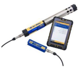
The AquaTROLL 500 MP handheld instrument has a combined pH/ORP sensor and other sensors for temperature, conductivity, pressure, and dissolved oxygen. The completely submersible sensor-equipped probe is connected to the rechargeable power pack. Sensor readings are transmitted by Bluetooth from the power pack to the Android or iOS tablet/smart phone. The unit uses In-Situ's VuSitu app to collect the data.
