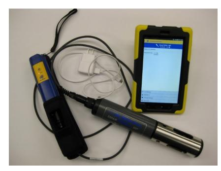
The smarTROLL MP handheld instrument has a combined pH/ORP sensor and other sensors for temperature, conductivity, pressure, and dissolved oxygen.
