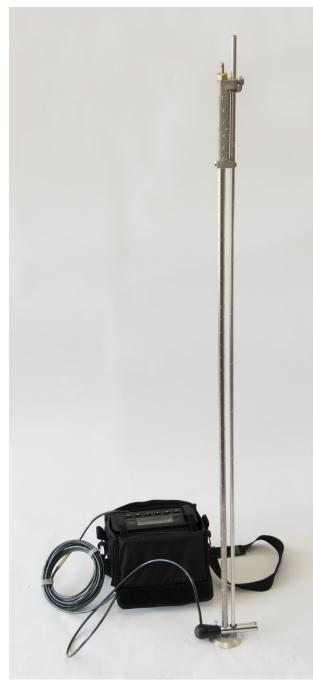
The Marsh-McBirney Model 2000 Flo-Mate uses an electromagnetic sensor to measure water velocity. Powered by two D-size batteries, the unit has a measurement range of -0.5 to +19.99 feet per second (-0.15 to +6 meters per second). The top-setting wading rod allows the sensor to be conveniently set at 20%, 60%, and 80% of total depth.
