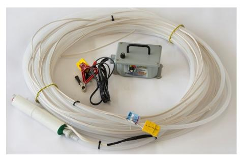
Mega-Typhoon is a 12 VDC two-stage submersible pump that has 80 feet of 3/8-inch ID HDPE tubing (tubing volume is 0.6 gal). The plastic pump body measures 1.7-inch OD by 10-inch length. Used with the Low Flow with Power Booster controller, the pump will produce 3.5 gpm at 10 feet of head and 0.25 gpm at 80 of head.
