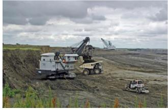
**Photo:** A dragline and shovel removes overburden and loads coal at the Falkirk Mine, North Dakota.
