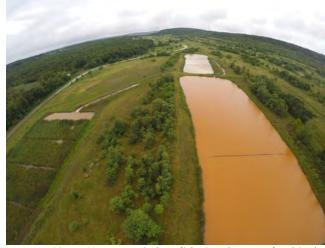
**Photo:** Unmanned Aircraft System image of acid mine drainage treatment ponds at the Flight 93 National Memorial in Pennsylvania.
