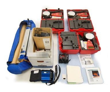
The Leica RTK 500 GPS survey system is a high-accuracy GPS/GNSS system for field surveying and data/point collection. The system consists of:
