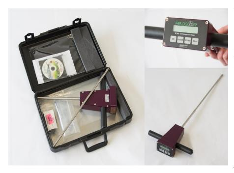
The portable soil compaction meter uses a cone penetrometer to measure soil compaction to a depth of 18 inches. The unit has a datalogger function that allows measurements to be downloaded to computer. The unit can also log GPS location Bluetooth using a connection to appropriate GPS unit.
