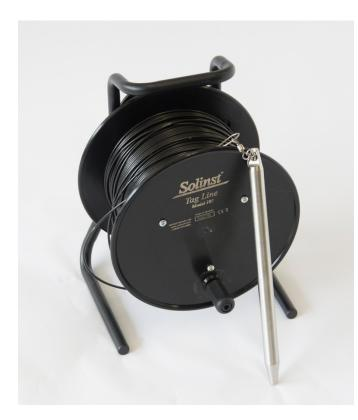
This tag line has a 500-foot polyethylene coated, permanently marked stainless steel cable clipped to a <sup>3</sup>/<sub>4</sub>-inch stainless steel weigh. The tag line is wound on a 10-inch diameter plastic reel with a brake. Every foot is labeled, and additional cable markings are at every <sup>1</sup>/<sub>4</sub> foot.
