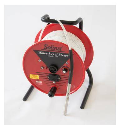
The water-sensing probe is attached to a 300-foot polyethylene flat tape with permanent markings every 1/100 of a foot. A dial allows the buzzer to be adjusted or turned off when the probe is in cascading water and ensures a clear signal when the probe contacts high- or low-conductivity water. The tape is wound on a 10-inch diameter plastic reel with a brake.
