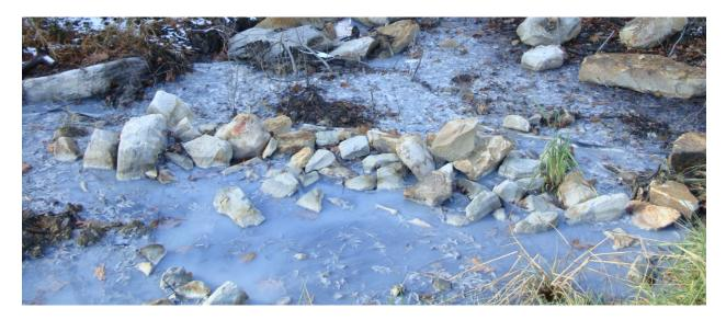
Figure 22: The milky-white water flowing out of a Bioreactor and through an outlet protection structure contains both elemental sulfur and calcite.
