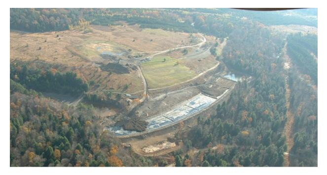
Figure 13: Bio Mix being spread over top of a non-woven geotextile and synthetic liner system during the construction of a 2.0 acre Bioreactor.
