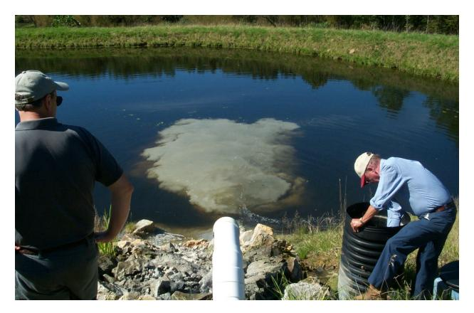
Figure 11: Short term flush of a Bioreactor effluent pipe to prevent build up of precipitates. Whitish elemental sulfur flushed into a subsequent pond filled with ferrous monosulfide. FeS particulates constantly discharge from this bioreactor to the settling pond due to an insufficiently sized Bio Mix layer.
