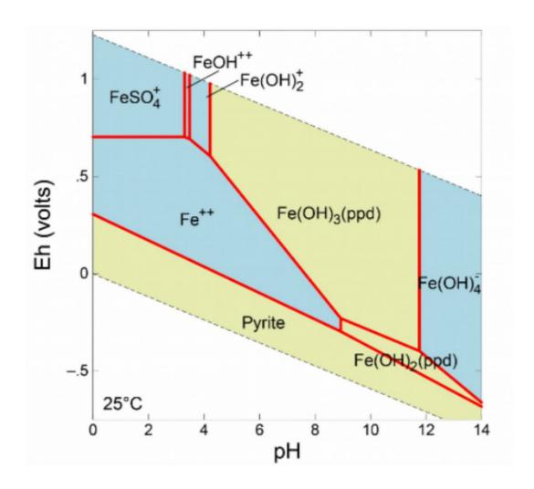
Figure 12.  $Fe(OH)_3$  solubility diagram with pH versus Eh. If water in the limestone layer contains any oxygen, ferrous iron will oxidize and precipitate as the pH increases > 6.0.
