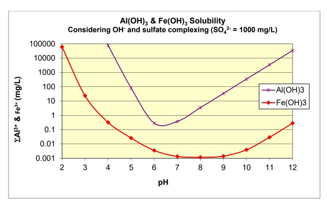
Figure 11: Aluminum becomes insoluble at pH > 5.5 and will precipitate and accumulate in the limestone. Ferric iron becomes insoluble at pH > 4.0.
