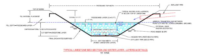
Figure 3: Typical Cross Section View of a Limestone Bed (LB) without a water layer.
