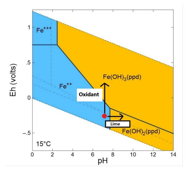
Figure 2. Eh – pH diagram illustrating the contrasting approaches of pH adjustment treatment strategy (lime or other alkali chemical addition) vs. an Eh adjustment treatment approach (permanganate or another oxidant). The blue areas of the diagram indicate stability fields where the dominate form of iron is dissolved. The tan areas of the diagram indicate Eh and pH conditions where iron is precipitated from solution.
