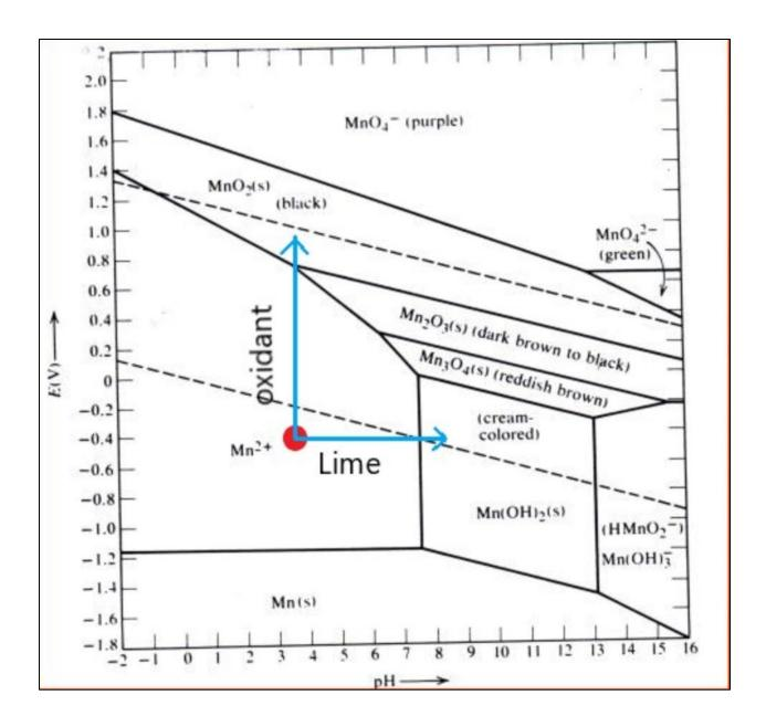
Figure 3. Pourbaix Diagram for Manganese with added arrows for either Lime addition or permanganate (oxidant) addition.
