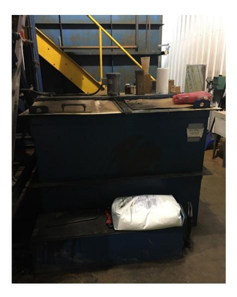
Figure 4. Mix Tank for a Potassium Permanganate treatment system.
