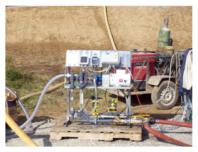
Figure 1: Blending skid with progressive cavity pump and computerized controls for emulsion polymer used at a site for flocculating iron hydroxide sludge and dewatering in Geotubes.
