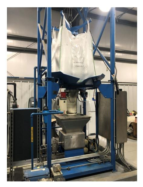
Figure 3. Super sack (1,650 lbs) feeder option as part of an automatic dry polymer make down system that automatically dispenses dry polymer product to produce a made down solution.
