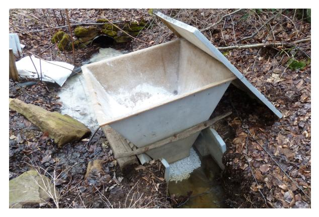
Figure 2. Photo of a soda ash dispenser with soda ash briquettes placed within mine drainage flow path.
