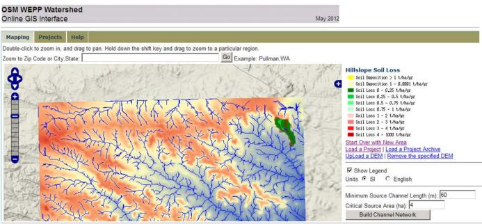
ABOVE FIGURE: A user-specified DEM and the soil loss map simulated with WEPP-Mine
