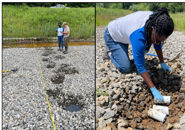
Figure 9. Emplacement of experimental reaction chambers by Ph.D. student Tashane Boothe-Lordon and co-I Dr. B. Hedin. Left: pH gradient within the Sterrett AMD limestone treatment bed is tested along the flow path. Right: Boothe-Lordon emplaces test precipitation chambers near the AMD inflow.
