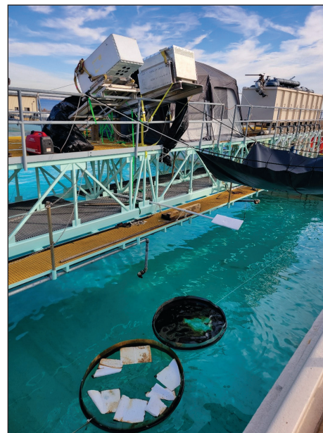
The LiDAR system was mounted on the auxiliary bridge above targets containing weathered crude oils to collect data.
