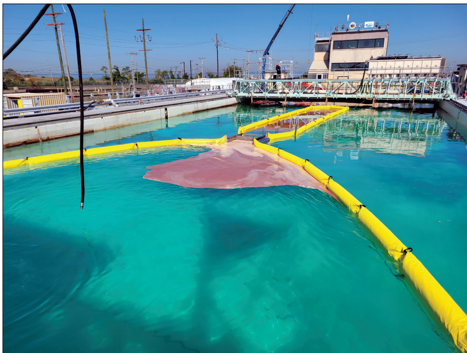
A new boom technique called the Restricted Burning Tongue is designed with a gate (fire break) at the mouth of the boom leading to a rigid stem of the fire boom to provide a controlled area for burning.
