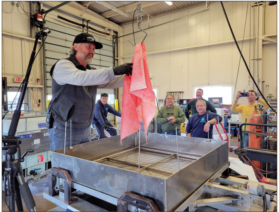
Using load cells to document weight changes at set intervals, the team also measured the final tear force of the sorbents.
