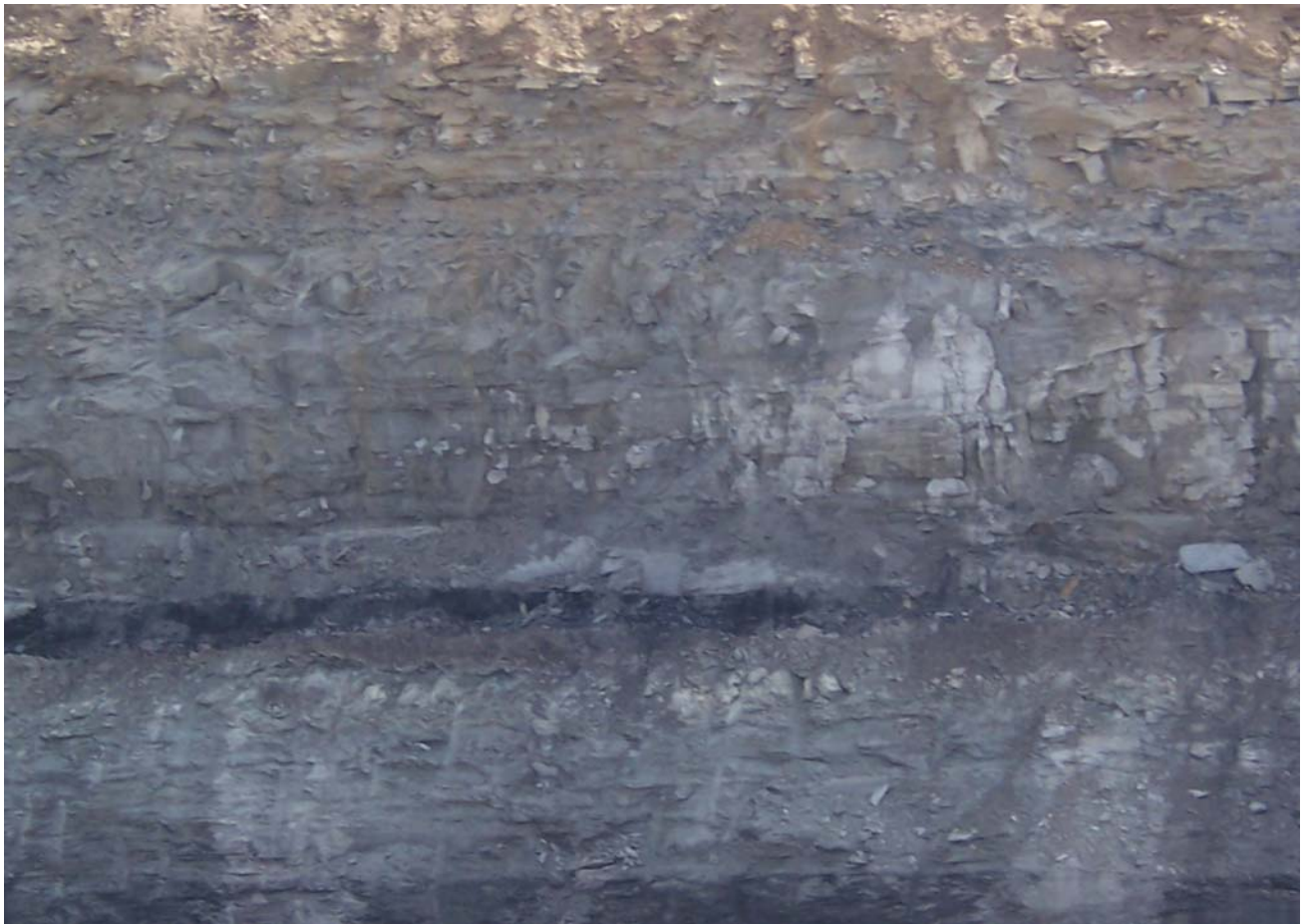
Coal seam in the rock highwall (dark layer about 1/3 from the bottom).
