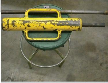
ABOVE PHOTO: This is a photograph of the Dynamic Cone Penetrometer.
