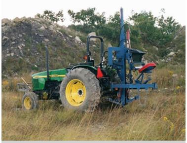
ABOVE PHOTO: This is a photograph of the Static Cone Penetrometer.
