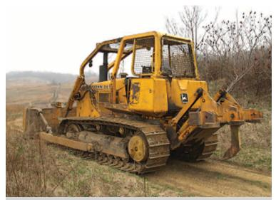
ABOVE PHOTO: D-6 sized dozer equipped with 36-inch ripping bar.
