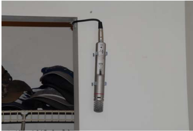
Figure 1.4 One (1) of 4 acoustic microphones located inside the House.
