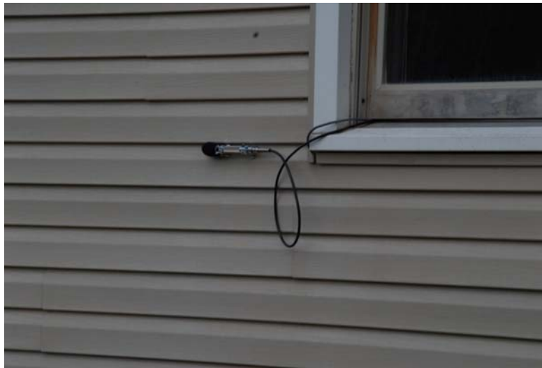
Figure 1.5 Airblast microphone located outside the House.
