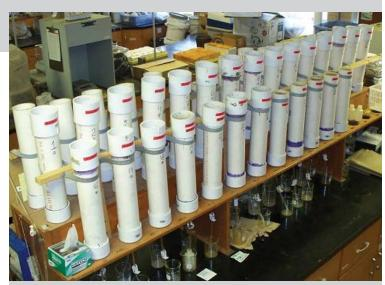
ABOVE PHOTO: Photograph of leaching column design used in this study. The columns were dosed twice weekly with 2.5 cm (1 inch) of simulated rainfall under both saturated and unsaturated conditions. Leachates were drained into the bottles/beakers on the bench below, but a water filled portion was maintained above the hose clamps to prevent gas exchange.
