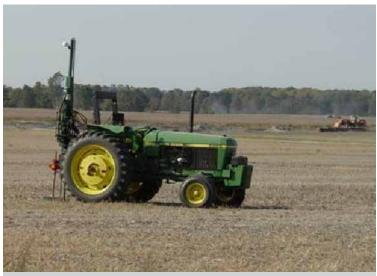
ABOVE PHOTO: Collection of cone penetrometer test measurements at the Lewis Mine site in Indiana.
