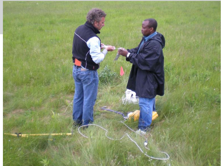
ABOVE PHOTO: Researchers collecting soil gas samples for isotope sampling during flux measurement.
