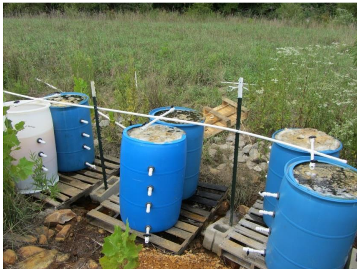
Test bioreactor cells (blue) and the limestone-only control (white) installed within the Tab-SImco full-scale bioreactor's inlet waterway.
