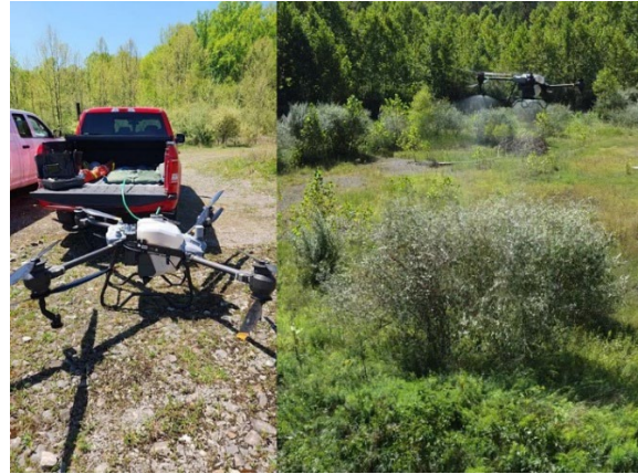
Uncrewed Agricultural Aerial System Tank Refill (Left) Aerial Herbicide Application (Right)
