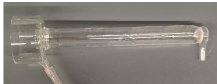
Fig. 18. The Patridge-Smith micro-flotation cell used in the flotation experiments.
