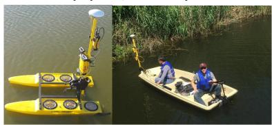
The bathymetric survey system can be mounted on the remote-control SeaFloor Systems Hydrone boat, or mounted on MCR's jon boat in order to produce 3D models of underwater terrain such as the bottom of water impoundments and sediment ponds. The system allows sites containing water features to be fully mapped by combining LiDAR or other surface elevation data with the underwater survey data.
