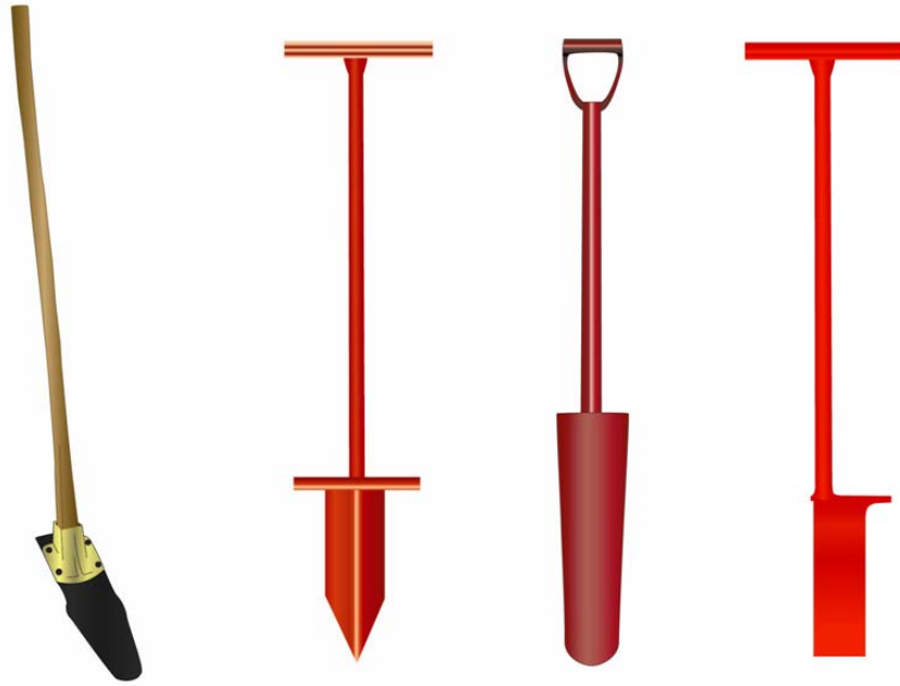
Figure 1. Four tree-planting tools that are used commonly on mine sites, from left to right: Hoedad, KBC planting bar, sharpshooter spade, and dibble bar.
