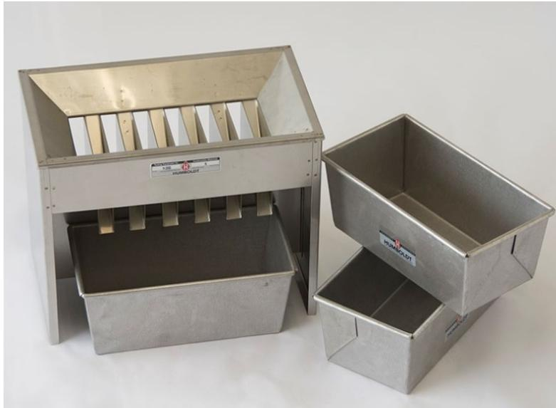
This 14-inch-long stainless-steel sample splitter has a removable hopper constructed of 12 chutes that discharge alternately to front and back. Chutes are  $\frac{3}{4}$  inch wide. Two pairs of cold-rolled steel pans come with the unit.
