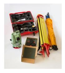
The Leica Total Station is a high-accuracy, reflector less field surveying and data/point collection device.
