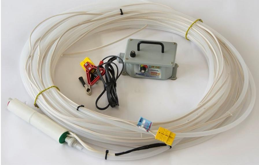
Mega-Typhoon is a 12 VDC two-stage submersible pump that has 80 feet of 3/8-inch ID HDPE tubing (tubing volume is 0.6 gal). The plastic pump body measures 1.7-inch OD by 10-inch length. Used with the Low Flow with Power Booster 1 controller, the pump will produce 3.5 gpm at 10 feet of head and 0.25 gpm at 80 of head.
