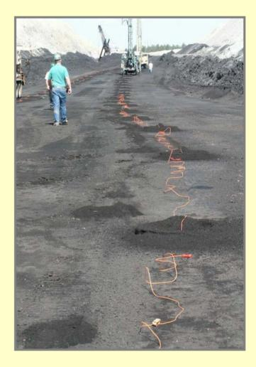
Many shock-tube system configurations are available from most explosive manufacturers. Ms trunkline delay assemblies are used for surface blasting. Many varieties of shock-tube delay detonators are available with a delay unit attached to one end of the tubing. Such a configuration can be used to generate individual-hole delays in a modified-series hookup.
