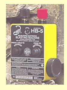
The blasting circuit in an electric-blasting system consists of electric detonators that are wired by connecting wires to the lead or firing line, which in turn is connected to the blasting machine.
