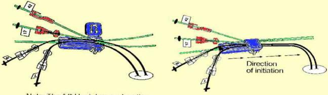
Note: The "J" Hook has no function in an all shock tube hook-up.
