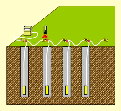
Precise timing control is the main advantage of electronic detonators. Detonator firing errors are on the order of microseconds, as distinguished from the ms errors associated with pyrotechnicdelay detonators. Electronic detonators use circuit boards and programmable applicationspecific integrated circuit (ASIC) processors to add very precise delays that are more reliable than traditional pyrotechnic delays.
