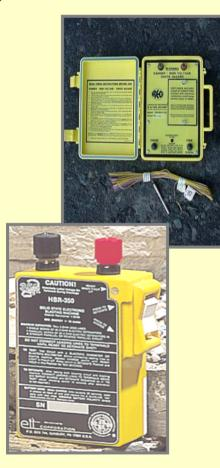
The lead (firing) line should not be laid out until the blast circuit is completely wired and all unnecessary personnel have been cleared to a safe location. After the lead line is laid out, it should be tested with a blaster's multimeter for continuity.
