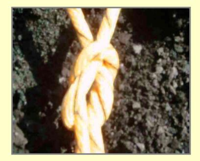
As a trunkline, detonating cord is used to initiate surface-delay units such as msdelay connector detonators, trunkline delays, and downlines.
