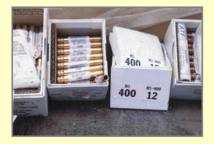
A **safety fuse** is a medium through which flame is continuously conveyed at a relatively uniform speed to initiate the heat-sensitive charge in an ordinary blasting cap. Cap-and-fuse assemblies are able to fire single charges or multiple charges designed to initiate in rotation.
