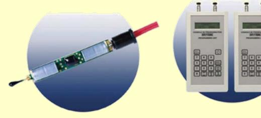
Simple systems use factory-programmed electronic detonators that are initiated from shock tubes in the same way that ordinary shock tubes detonate. Each of these electronic detonators contains a piezoceramic device and a timing oscillator.
