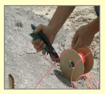
Detonating cord can be used as **downlines** or **trunklines**. As downline, detonating cord is used to initiate cord-sensitive boosters or ms-delay detonators.
