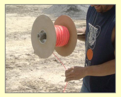
A general rule when selecting detonating cord is to use the lowest cord load possible consistent with conditions at hand.
