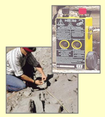
**Initiator** is a term used in the explosive industry to describe any device that may be used to start a detonation or a deflagration. There are four general classifications of initiators currently being used in surface coal-mine blasting:
