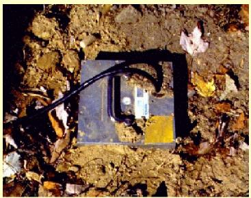
The longitudinal channel should be pointing directly at the blast and the bearing should be recorded
