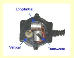
Inside housing showing transducer orientations
