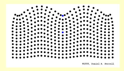
Ground vibrations are measured in terms of **particle** *velocity* and are reported in inches per second (ips) or the speed at which a particle of soil or rock moves.
