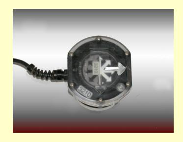
Where access to the structure and/or property is not available, the sensor should be placed closer to the blast in undisturbed soil.
