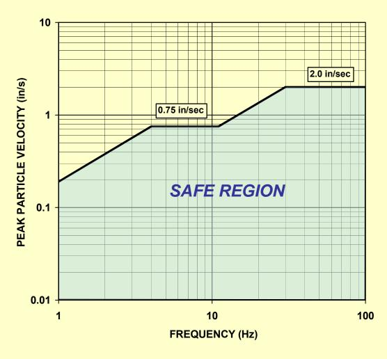
Figure 1.—Modified Blasting Level Chart
