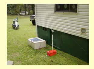
If placed too close to a structure, the airblast may reflect from the house surface and record higher amplitudes.
