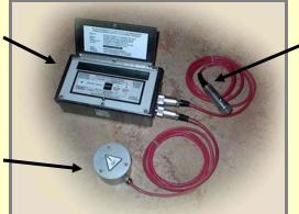
a microphone or airblast sensor.
