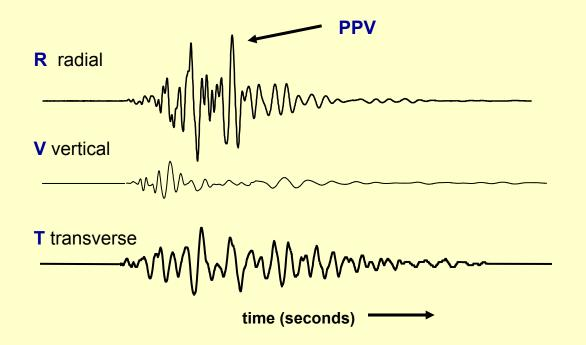
The time history is made up of peaks and troughs of motion, the height of any wave is the amplitude.
