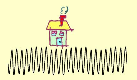
High frequencies do not promote structure shaking. The length of a single high-frequency wave cycle is short as compared with the dimension of a structure. A structure does not significantly respond to high frequencies.
