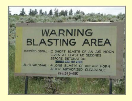
Signs that state "Warning! Explosives in Use" must also be placed at all entrances, from public roads or highways, to the permit area. Such signs must both clearly list and describe the meaning of the audible blast warning and all-clear signals that are in use and explain the markings of blasting areas and charged holes awaiting firing within the permit area.
