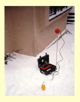
The sensor should be placed on or in the ground on the side of the structure towards the blast. A structure can be a house, pipeline, telephone pole, etc.
