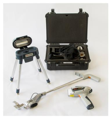
The Niton XL3t 950 GOLDD+ handheld analyzer is a portable elemental analysis tool that will detect elements with an atomic number 12 or above and will present a spreadsheet with the measured elements in either parts per million or as a percentage of the material being tested.
