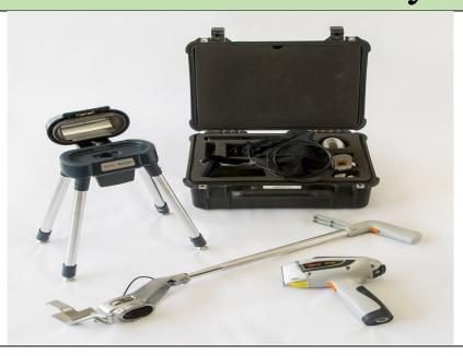
**Description:** The Niton XL3t 950 GOLDD+ handheld analyzer is a portable elemental analysis tool that will detect elements with an atomic number 12 or above and will present a spreadsheet with the measured elements in either parts per million or as a percentage of the material being tested.
