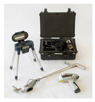
The Niton XL3t 950 GOLDD+ handheld analyzer is a portable elemental analysis tool that will detect elements with an atomic number 12 or above and will present a spreadsheet with the measured elements in either parts per million (ppm) or as a percentage (%) of the material being tested.
