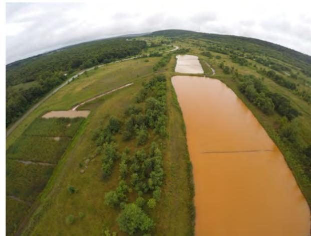
Photo: Unmanned Aircraft System image of acid mine drainage treatment ponds at the Flight 93 National Memorial in Pennsylvania.
