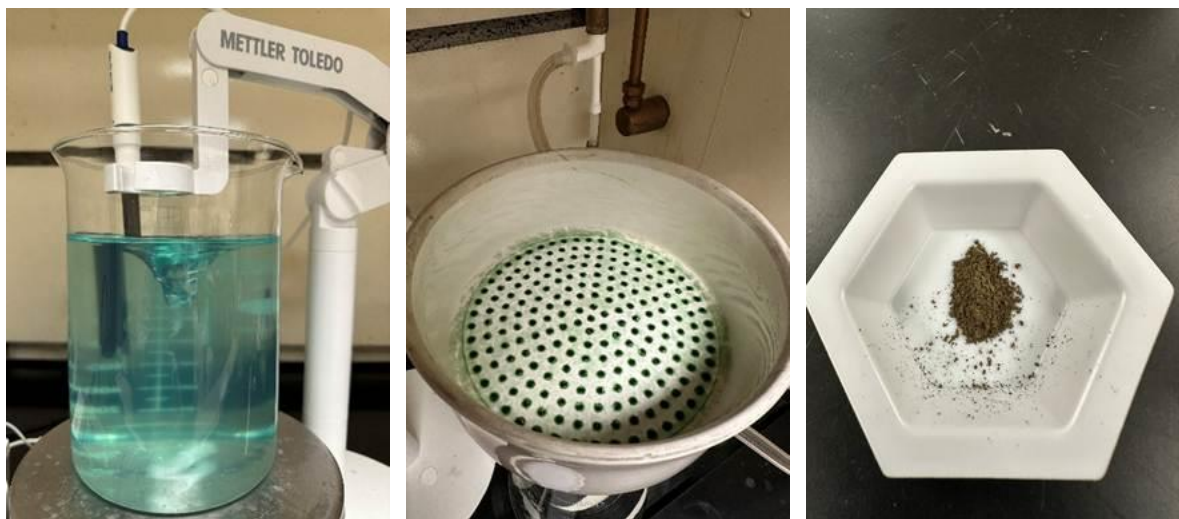
Figure 31. Cobalt Hydroxide Precipitation. Left: Enriched Solution + NaOH. Center: Solids Filtration. Right: Dried Solids.
