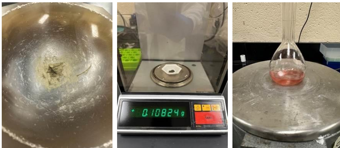
Figure 32. Cobalt Hydroxide Solids Digestion. Left: Mortar Mixing. Center: Weight of Digested Solids. Right: Solution During Digestion.
