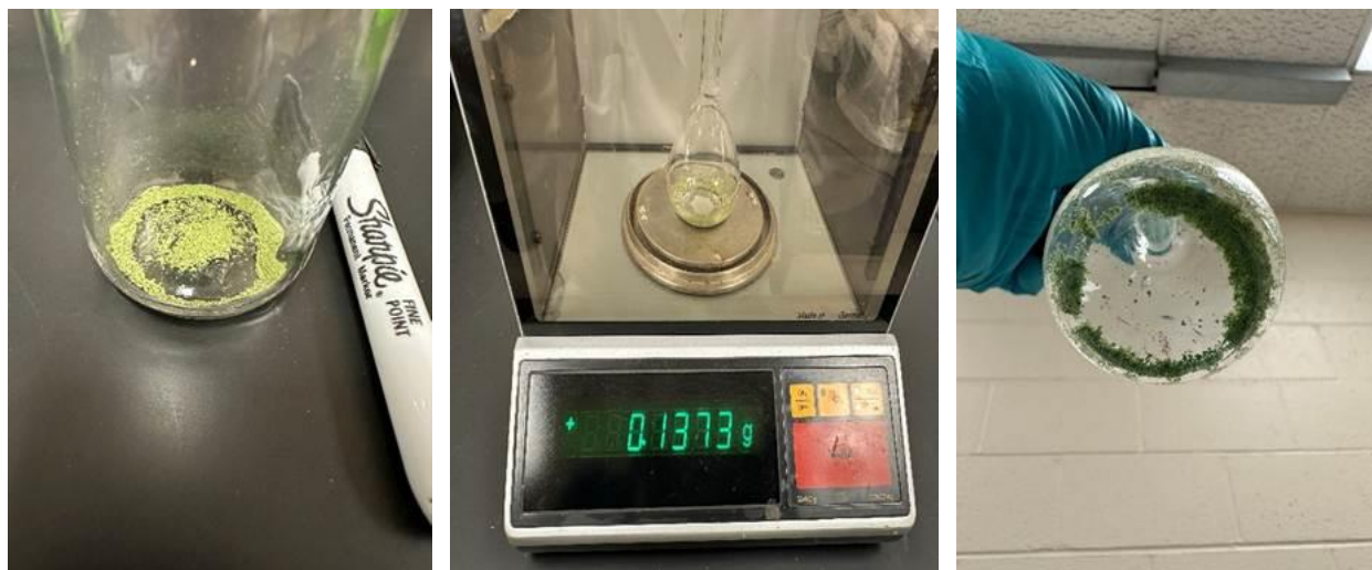
Figure 17. Nickel Hydroxide Solids Digestion. Left: Dried Solids. Center: Weight of Digested Solids. Right: Solids in Digestion Vessel.
