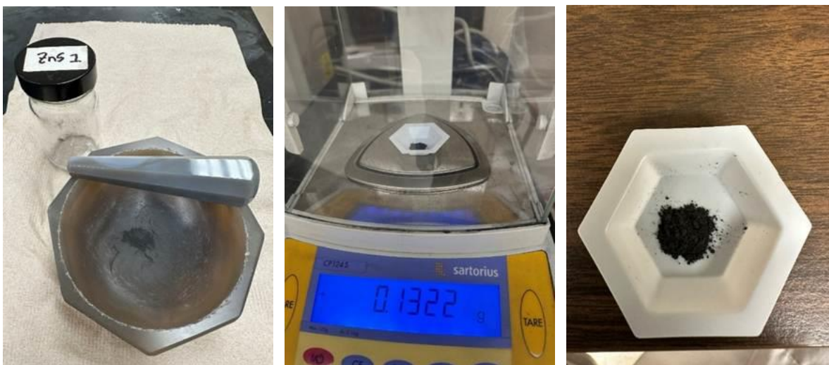
Figure 29. Zinc Sulfide Solids Digestion. Left: Mortar Mixing. Center: Weight of Digested Solids. Right: Solids for Digestion.
