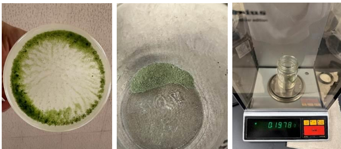
Figure 16. Nickel Hydroxide Precipitation. Left: Wet Solids. Center: Dried Solids. Right: Weight of Dried Solids.
