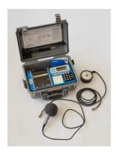
The portable seismograph system allows user to set up the unit in the field at the desired location (usually at a house near the blast site) and record ground vibration as well as sound (air blast) from blasting events. The unit also has a printer that allows for immediate display and printing of the blast events in the field. The print-out can be given to the homeowner at their home, if needed.
