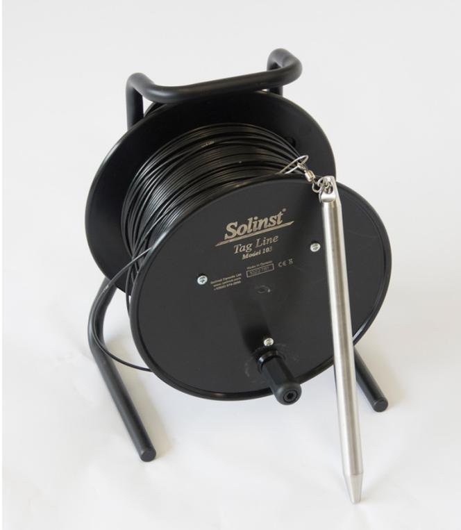
This tag line has a 500-foot polyethylene coated, permanently marked stainless steel cable clipped to a  $\frac{3}{4}$ -inch stainless steel weigh. The tag line is wound on a 10-inch diameter plastic reel with a brake. Every foot is labeled, and additional cable markings are at every  $\frac{1}{4}$  foot.
