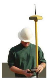
The Topcon Hiper+ is designed as a centimeter accuracy GPS solution to enable georeferencing for GIS-building, accurate control for remote sensing and precision navigation, among other uses. The system includes
