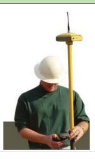
**Description:** The Topcon Hiper+ is designed as a centimeter accuracy GPS solution to enable georeferencing for GIS-building, accurate control for remote sensing and precision navigation, among other uses. The system includes:
