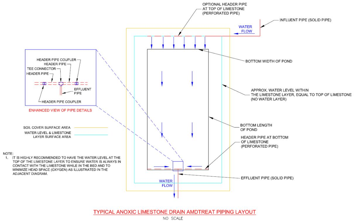
Figure 3: Plan View of the ALD to Illustrate Common Piping Layout and Components (Used in AMDTreat Piping Calculator) and the Layer Surface Areas
