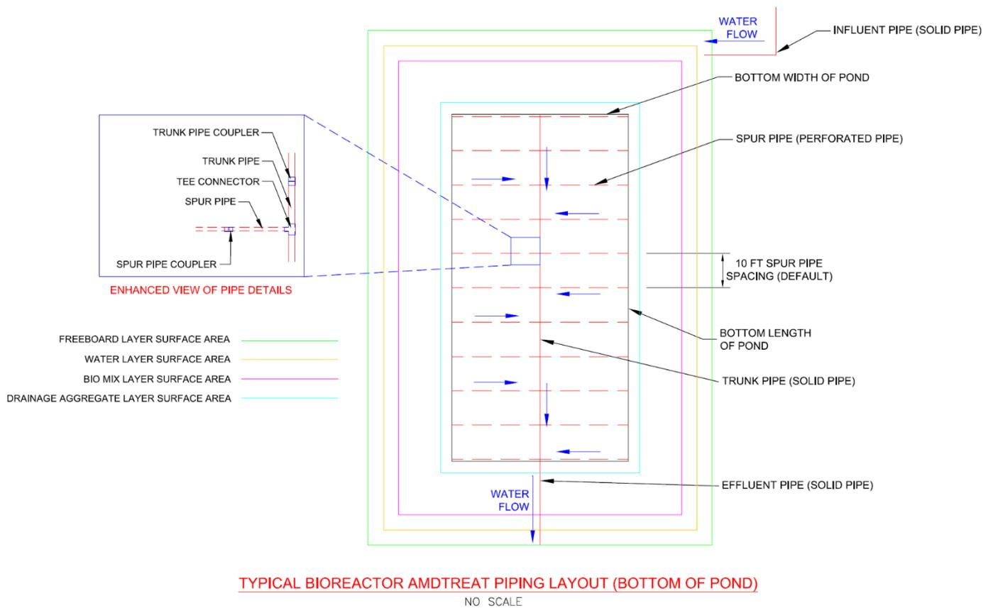
Figure 3: Plan View of the Bioreactor to Illustrate Common Piping Layout and Components (Used in AMDTreat Piping Calculator) and the Layer Surface Areas.
