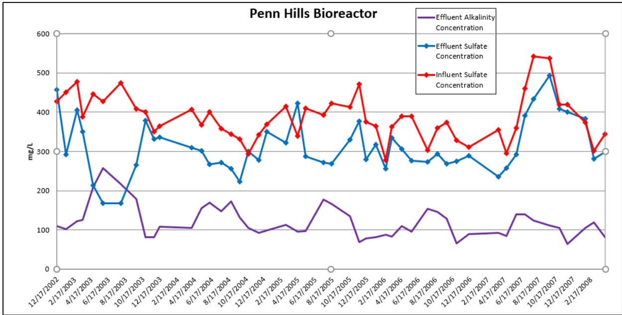
Figure 17: Monthly Influent and effluent sulfate concentration and effluent alkalinity concentrations for a Bioreactor over a five-year period.
