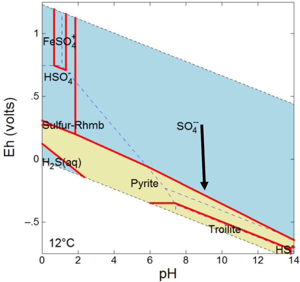
Figure 16: Pourbaix diagram for an aqueous iron/sulfur system. Most mine drainage would plot within the  $\text{SO}_4^{2-}$  stability field. The goal of a Bioreactor is to create an Eh/pH condition that plots in the pyrite stability field.
