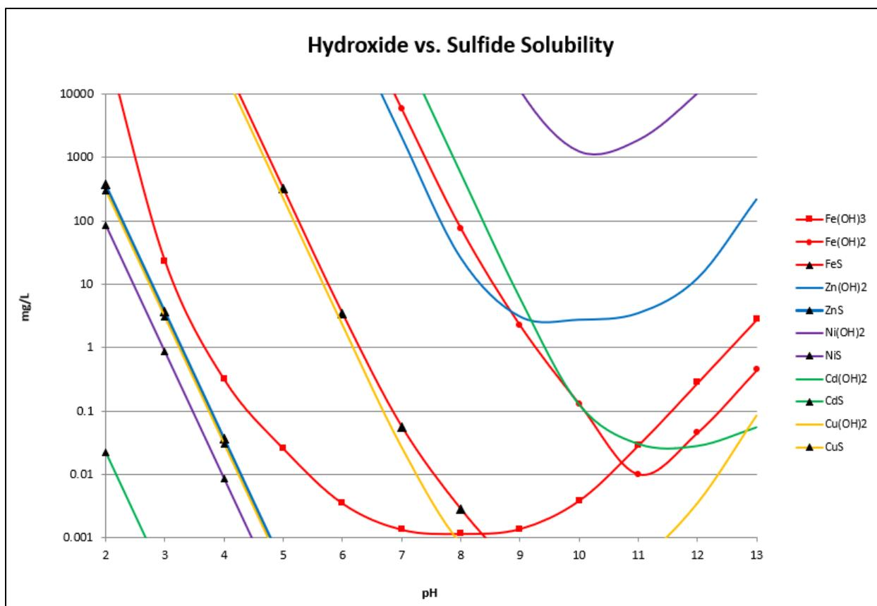
Figure 15: Solubility of metal hydroxide vs. sulfides for various elements
