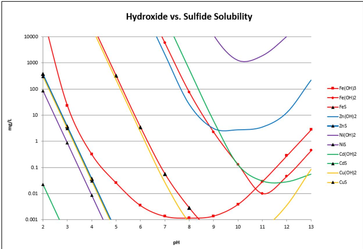
Figure 15: Solubility of metal hydroxide vs. sulfides for various elements
