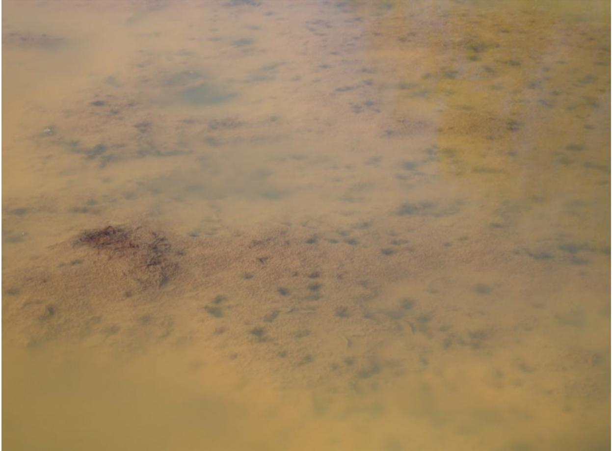
Figure 21: Photo showing a 3.0 by 3.0 ft area of the top of a Bio Mix layer under the water layer. One to two-inch diameter holes can be observed made by CO<sub>2</sub> produced in the Bio Mix layer. The pH 2.7 mine water entering the Bioreactor and low pH iron oxidization is causing a ferric hydroxy sulfate mineral crust on top of the Bio Mix layer.
