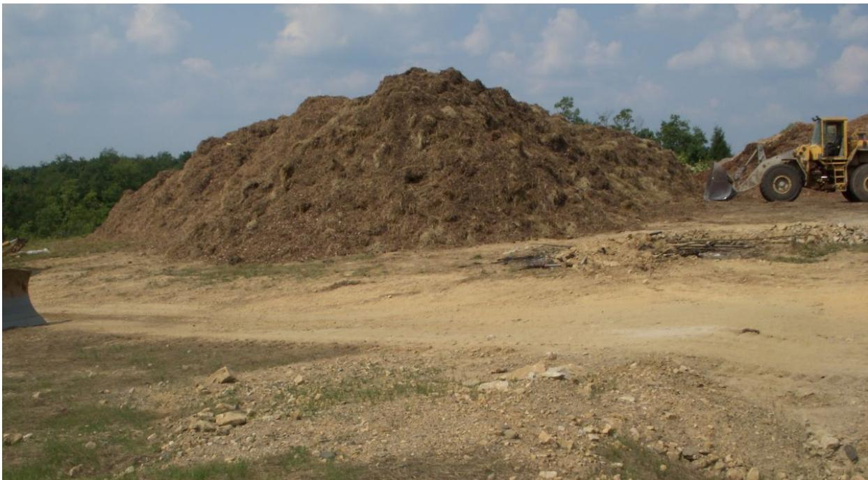
Figure 5: Large pile of Bio Mix (manure, compost, hay, woodchips, limestone) in preparation to be placed in Bioreactor.
