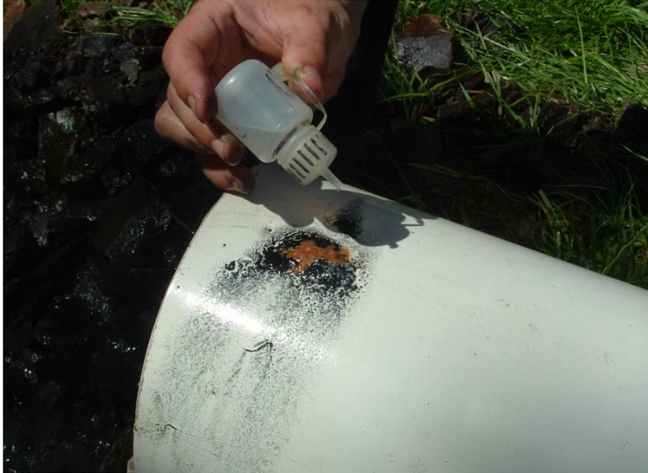
Figure 23: Black precipitate at the base of a bioreactor effluent pipe (black coated rocks to left of white pipe). Hydrogen peroxide is added to the black precipitate and the oxidation to produce an orange-red color ferric hydroxide confirms the precipitate as iron sulfide.
