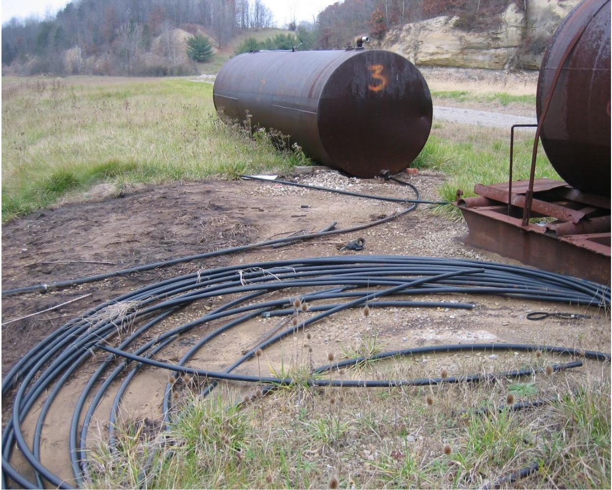
Figure 10: Steel Caustic Soda storage tank and poly feeder line. Note the lack of vegetation indicating a Caustic Soda leak.
