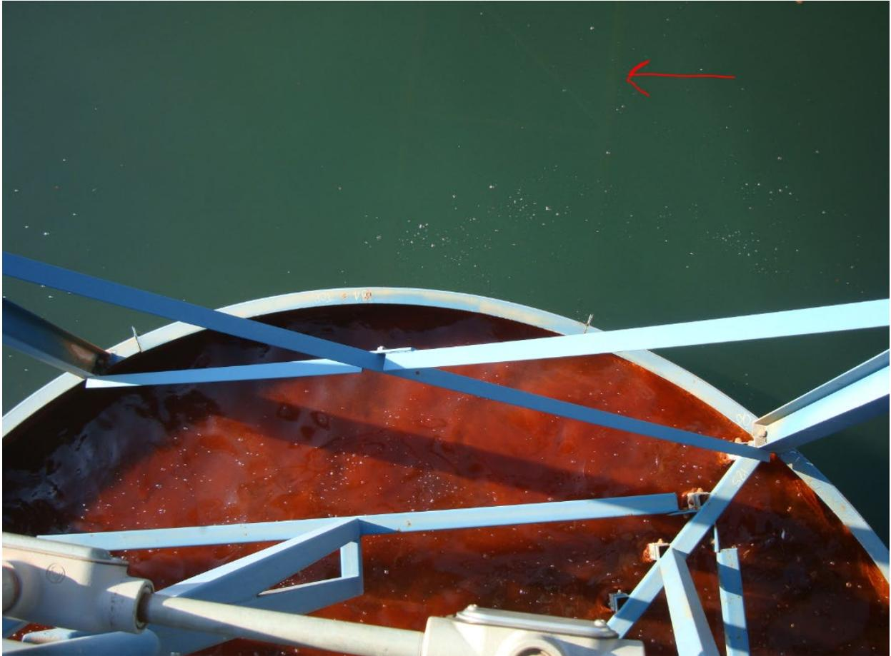
Figure 7: Example of a flocculating center well. Polymer flocculant is added to pH-adjusted mine drainage at a hydraulic jump in the conveyance trough. The center well is designed to dissipate flow velocity and promote agglomeration of particles. Note transport rakes, located 20 ft under the water surface can be seen (see red arrow).
