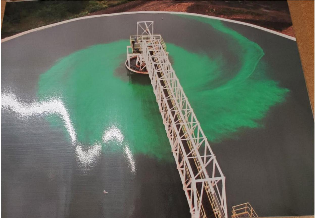
Figure 17: Dye test on a large 220 ft diameter steel clarifier. Note rotation caused by rake movement.
