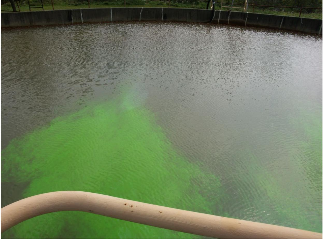
Figure 15: Dye showed a preferential flow path of water on one side of the clarifier that increased water velocity causing poor settling and turbid effluent. Metal baffles were welded into the center well to improve flow distribution. This created a radial flow path emanating from the center well and resulted in improved effluent clarity. into the center well to redistribute the watering flowing down through the clarifier.
