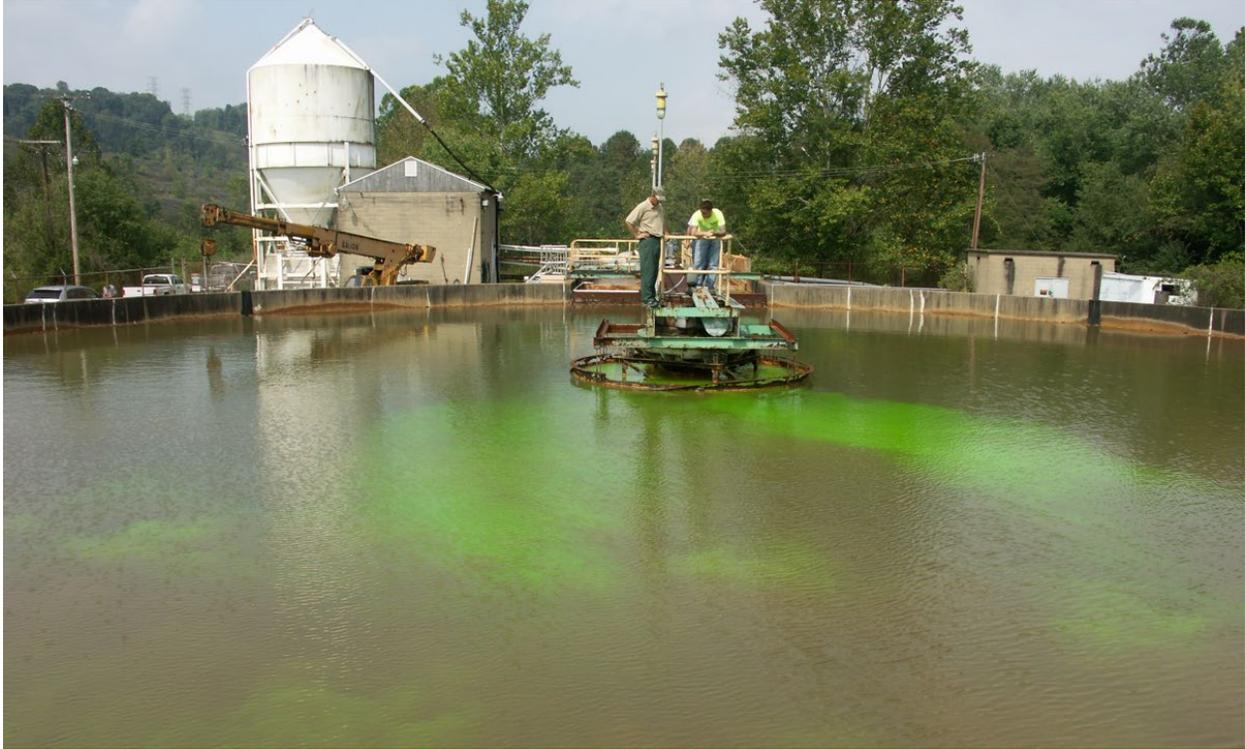
Figure 16: Alternative view of dye test shown in Figures 14 and 15. Before the installation of the flow baffle in the center well, dye preferentially flowed on one side of the clarifier.
