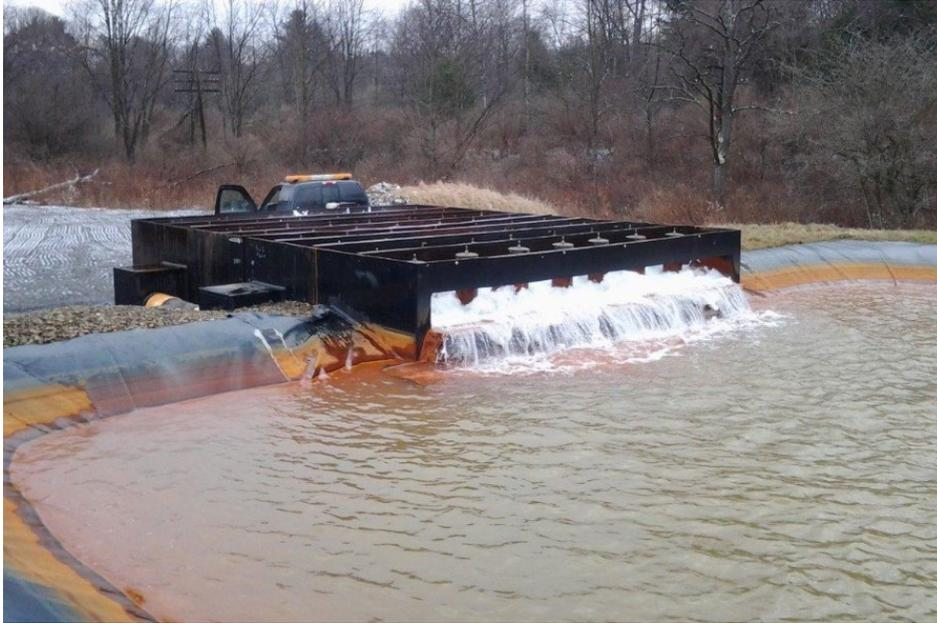
Figure 16: Maelstrom Oxidizer aerator unit used to decarbonate anoxic and carbonated underground mine drainage. Compressed air blower not visible in photos.
